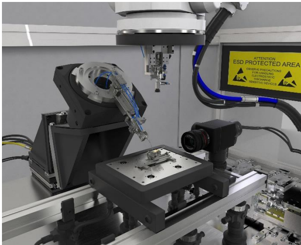
Figure 1: An application example is shown: an x- and y-positioner stacked with a goniometer (movement around z-axis) and a tilted rotator are used to align two fiber ends such that the light is coupled.
